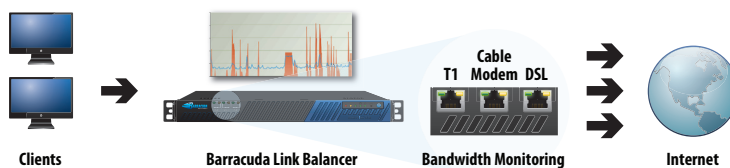
Figure 2. The Barracuda Link Balancer distributes traffic across multiple active Internet links
